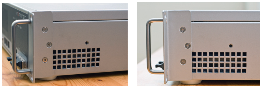
Figure 1: Installed mounting brackets
