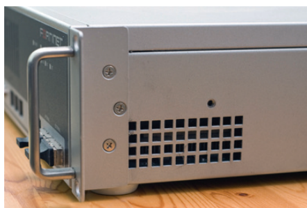
Figure 1: Installed mounting brackets
