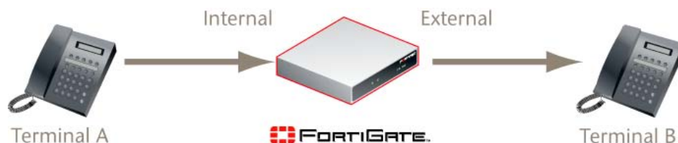
Figure 2: FortiGate unit in Transparent mode
