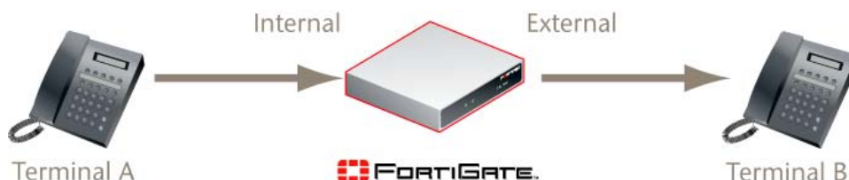
Figure 3: FortiGate unit in NAT/Route mode
