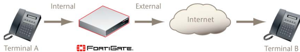
Figure 3: FortiGate unit in NAT/Route mode
