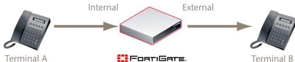
Figure 2: FortiGate unit in NAT/Route mode
