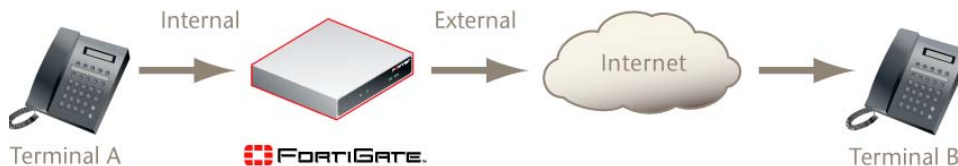
Figure 3: FortiGate unit in NAT/Route mode
