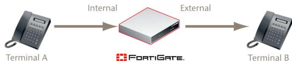
Figure 1: FortiGate unit in Transparent mode
