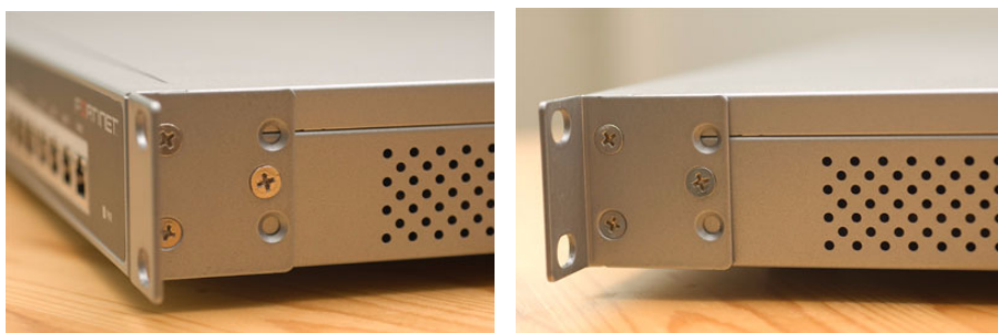
Figure 1: Installed mounting brackets
