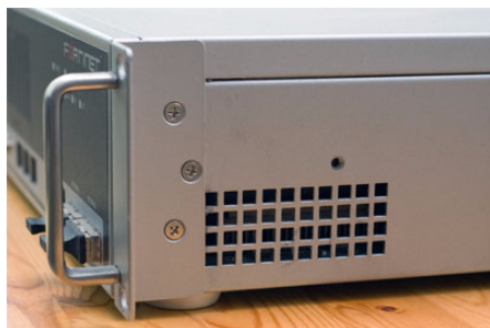
Figure 1: Installed mounting brackets
