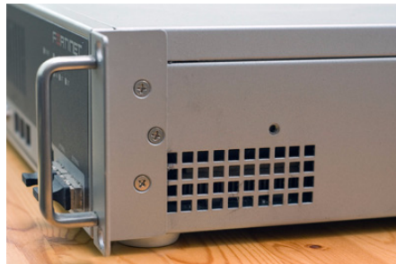
Figure 1: Installed mounting brackets
