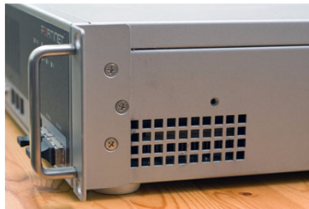
Figure 1: Installed mounting brackets
